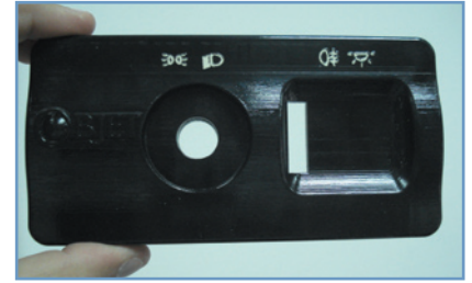
Step 9: Label PolyJet models with laser etching
