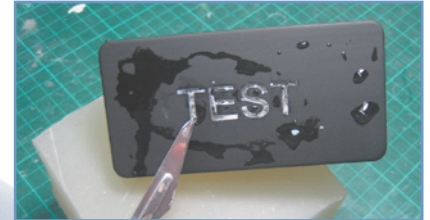
Step 6: Recessed Text – use scalpel or Waterjet
