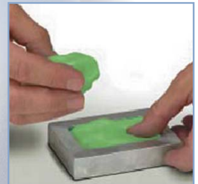
Figure 2: Placing the Objet model inside the mold
