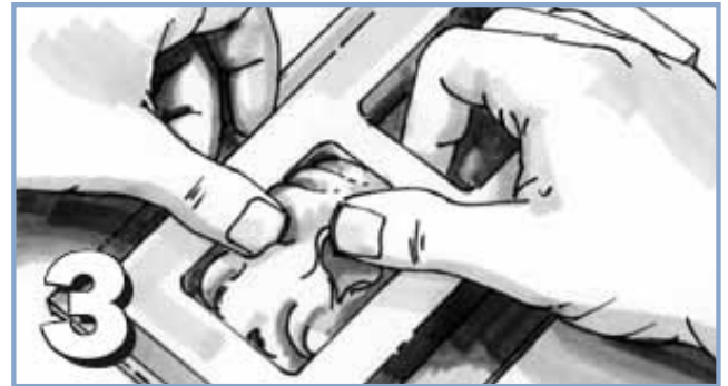
Placing and embedding the rubber onto model
