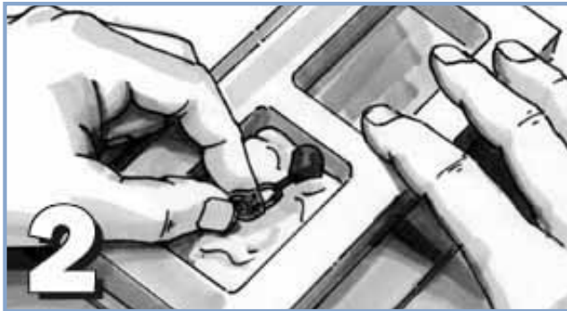
Place the Objet model inside the Silicone Mold
