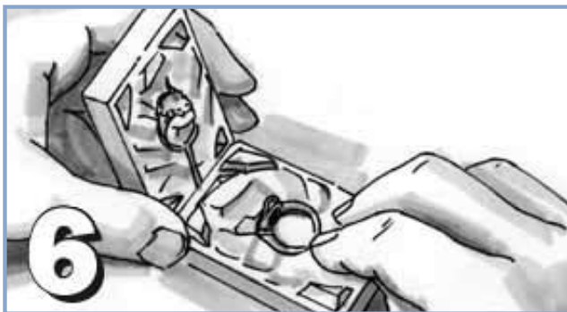
Parting lines are easily controlled and corrected by hand when used with the powder separation
