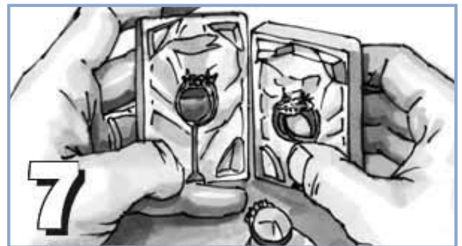
Finished molds can be complex with cores, straight plugs or even spiral plugs.
