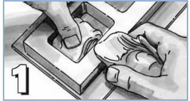
Silicone Molding Rubber is soft and pliable, with a consistency like putty or molding clay
