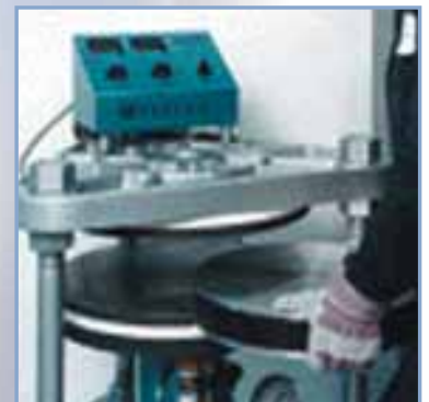
Figure 8: Vulcanizing The Mold
