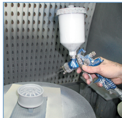
Figure 6. Apply Primer Paint.
