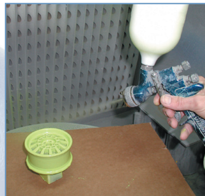
Figure 7. Apply Final Paint.
