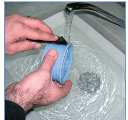
Figure 2. Wet-sanding. Wet-sand the model with 320-grid sandpaper.
