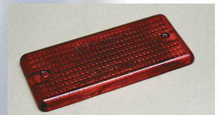
Figure 1: Remove support material Remove support material thoroughly with the WaterJet station. Optionally, remove any remaining residual material with a cleaner/degreaser (Zep Citrus Cleaner) if necessary
