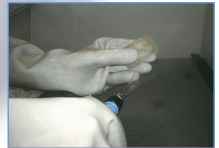
Figure 2. Wash model. Pressure wash the model to remove all support material.
