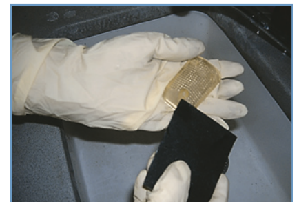
Figure 3. Dry-sanding the part. Sand all surfaces to smooth the model.
