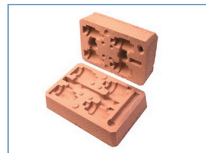
Picture 3. The sand casting mold – forming the cavity.
