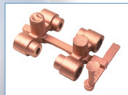
Picture 5. The desired bronze cast model.
