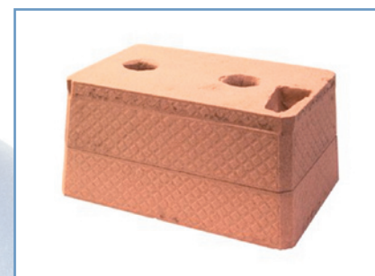
Picture 4. The pattern is removed from the flask.
