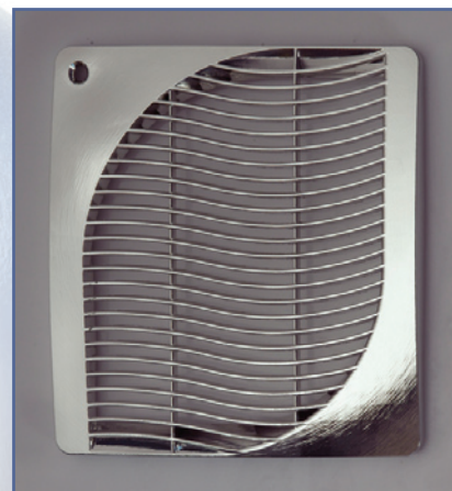
Picture 5. PolyJet model coated with chrome finish
