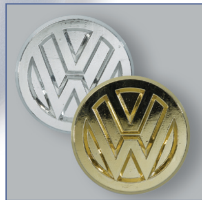
Picture 6. Vacuum metalizing samples
