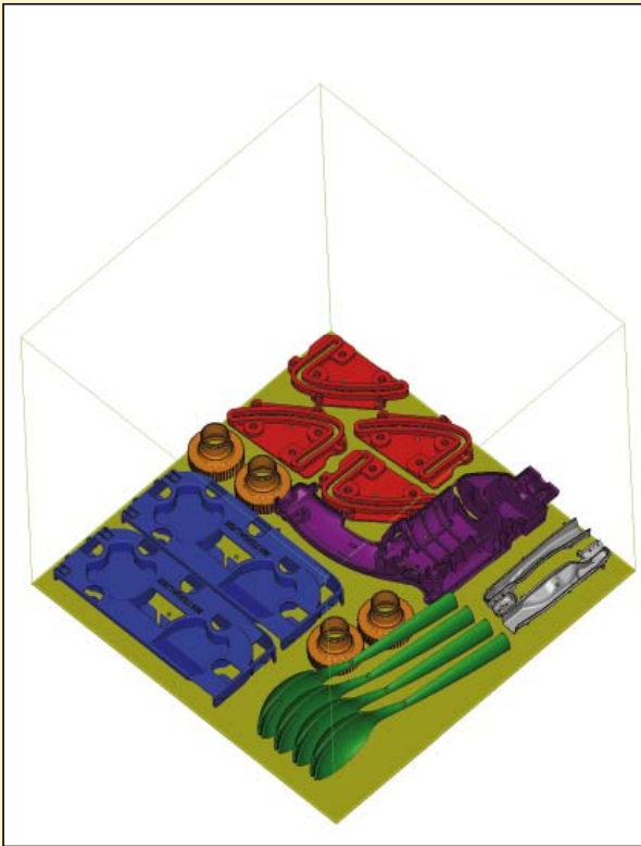
Maximise the number of parts on the build platform
